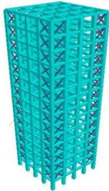
**Fig. 3.5(a) Structural Plan for X-braced RC Frame (Model-3)**
