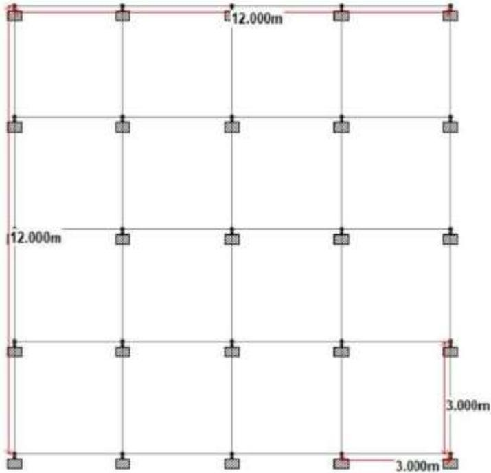
**Fig.3.2 Structural Layout of RC Frame Prototype**
