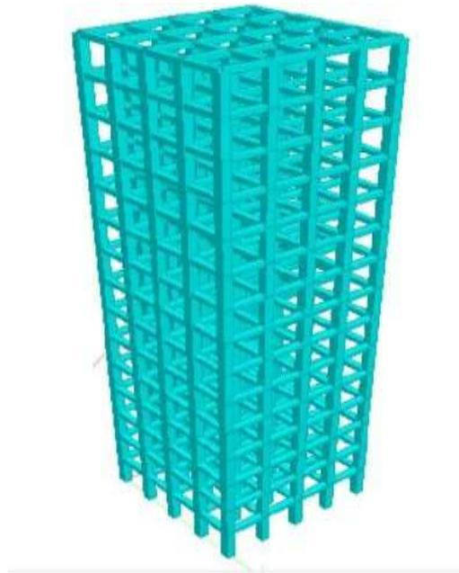
**Fig. 3.3(b) Rendered view of unbraced RC Frame (Model-1)**
