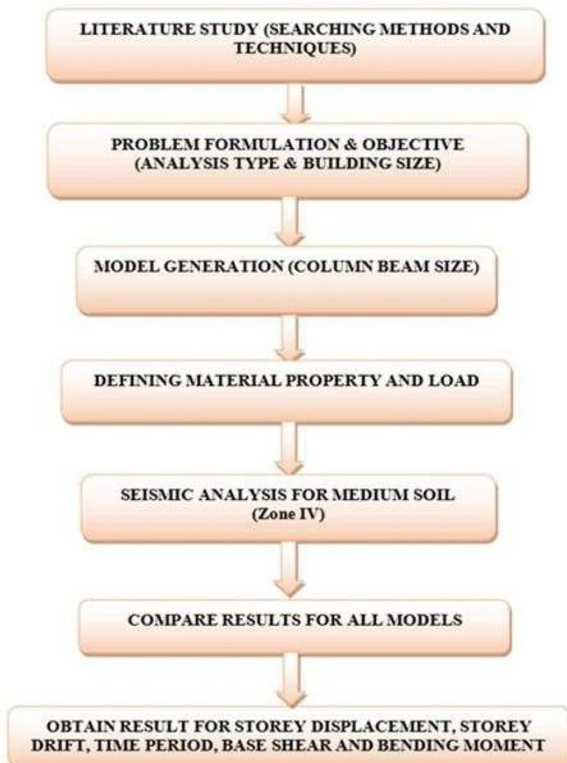
**Fig. 3.17 Flow chart of the analysis procedure**
