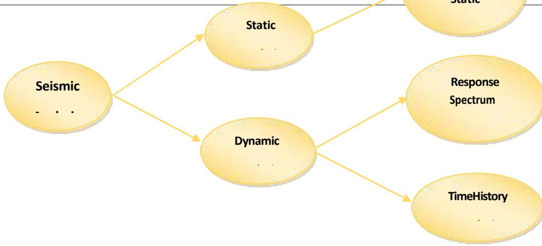
**Fig. 3.13 Classification of seismic analysis**
