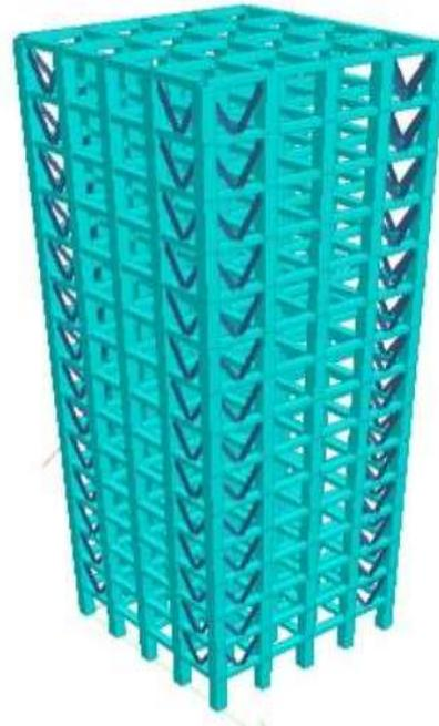
**Fig. 3.9(a) Structural Plan for V-braced RC Frame (Model-7)** **Fig. 3.9(b) Rendered view for V-braced RC Frame (Model-7)**
