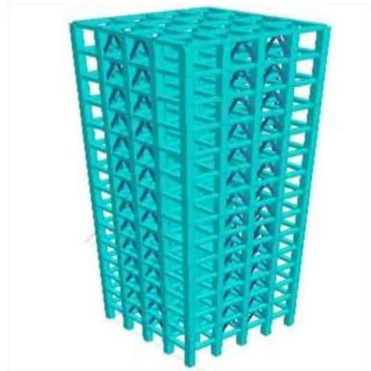
**Fig. 3.6(a) Structural Plan for Inverted V-braced RC Frame (Model-4)**
