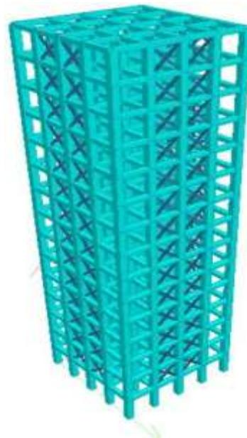
**Fig. 3.4(b) Rendered view for X-braced RC Frame (Model-2)**
