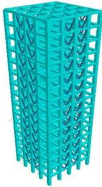
**Fig. 3.8(a) Structural Plan for V-braced RC Frame (Model-6)**
