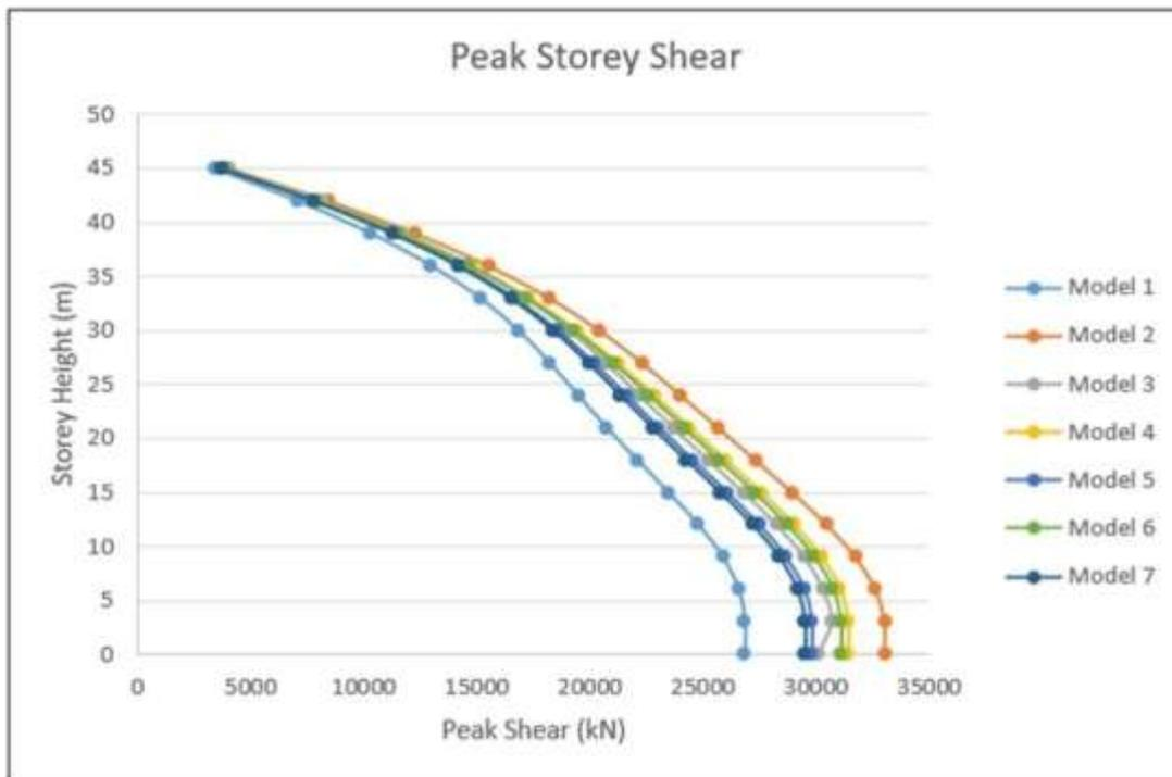
**Fig. 5.12 Peak storey shear for Different models**
