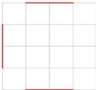
**Fig. 3.4(a) Structural Plan for X-braced RC Frame (Model-2)**
