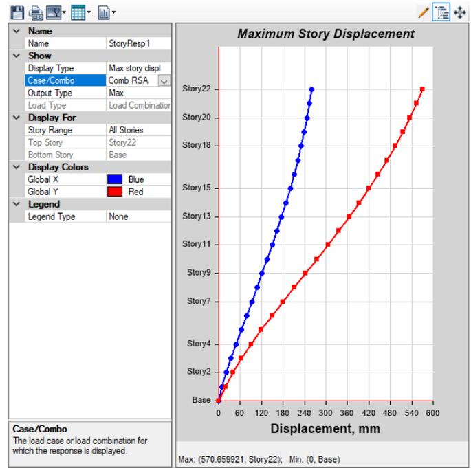
Fig. 5.1.6 Storey Displacements in MODEL-VI
