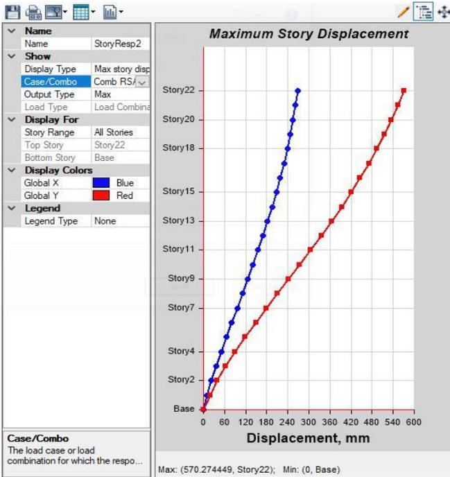
Fig. 5.1.5 Storey Displacements in MODEL-V
