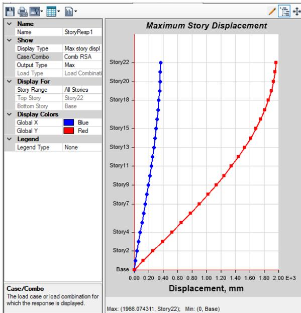
**Fig. 5.1.1 Storey Displacements in MODEL-I**
