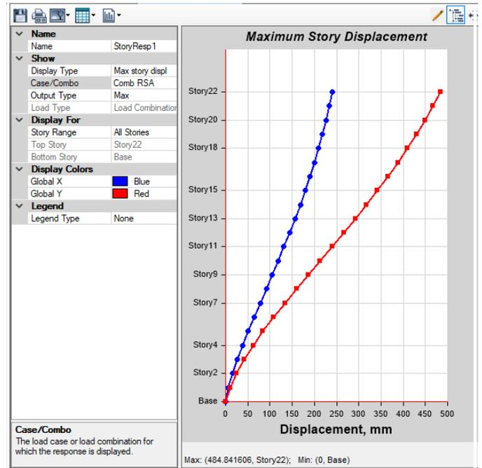
**Fig. 5.1.2 Storey Displacements in MODEL-II**
