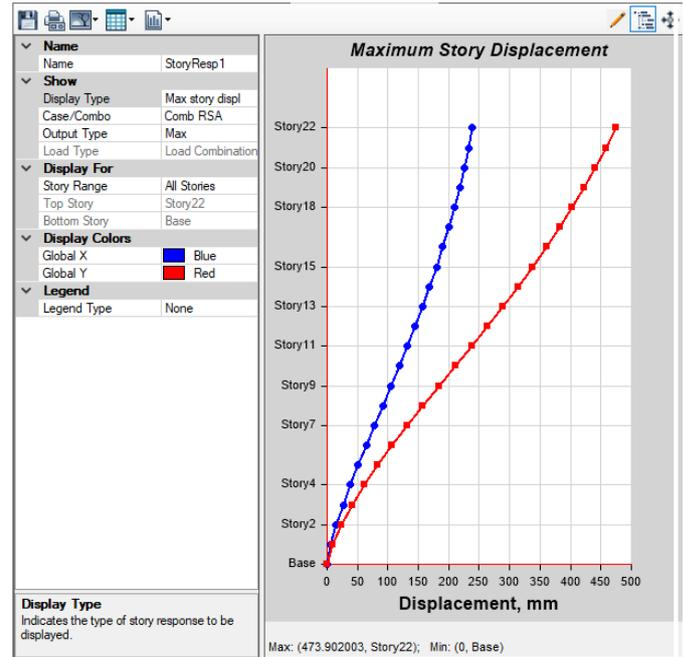
Fig. 5.1.4 Storey Displacements in MODEL-IV
