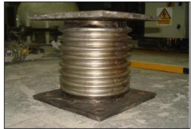
Fig. 1.4a Accordion Metallic Damper
