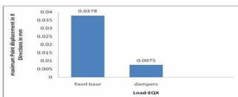
in case of fixed base and less in dampers. At all external and internal column points displacement was found to be less. Point displacement only checked at top story.
