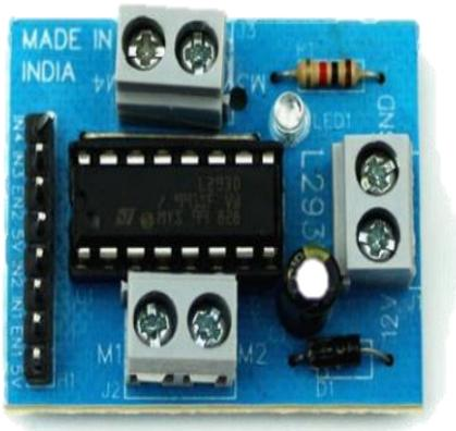
This module is used to drive DC motors. As the module uses dual H-bridge drive, it is possible to drive two motors at the same time. It supports driver voltage from 5v to 35v.
