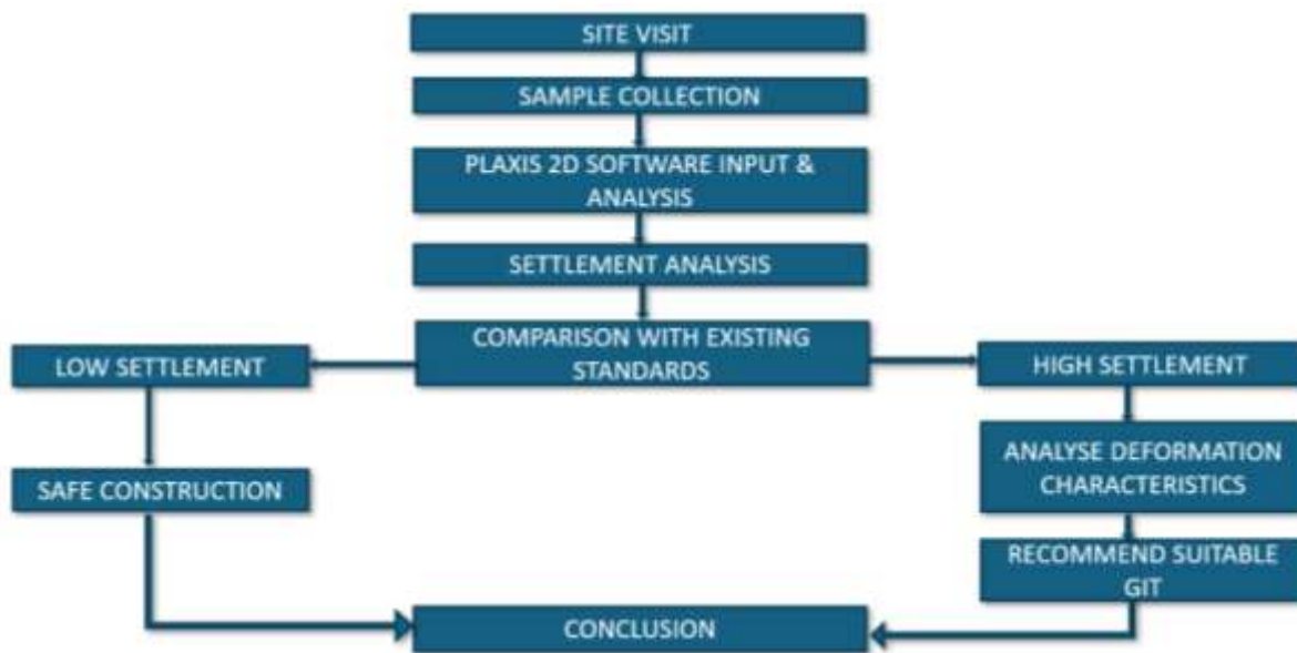
Fig. 3.1 Methodology adopted for settlement analysis of soft clay
