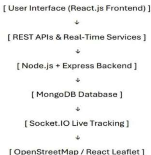
Fig. 2. Layered Client-Server Architecture of SHERISES
