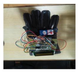
circuit. A 16/2 LCD display is also connected to the Arduino. The flex sensors gives the readings of the bending of the fingers. Depending upoun the bend of the fingers, Arduino gives the output on the screen. An accelerometer recognise the movement of the hand depending on the changes in the directions of X-axis, Y-axis and Z-axis.
