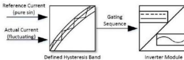
Figure 3. Block Diagram Hysteresis Current Control
