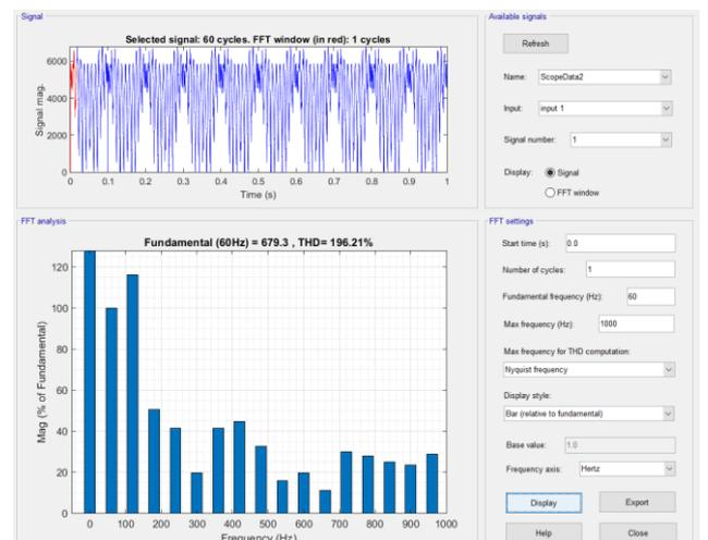
Figure. 8. FFT-Analysis of Load Current without filter
