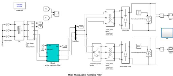
Fig. 5. Simulink Model of Three-Phase with SAPF
