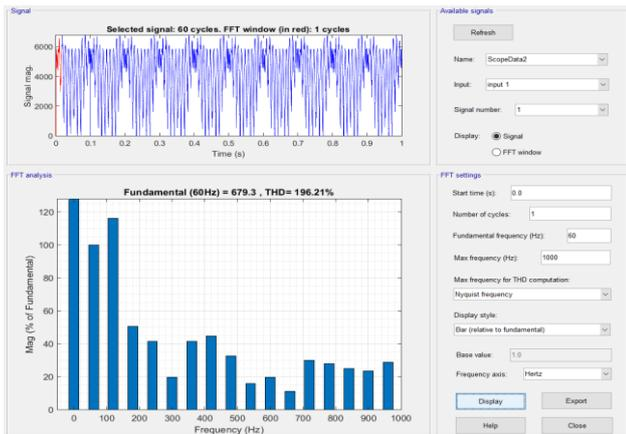
Figure. 8. FFT-Analysis of Load Current without filter
