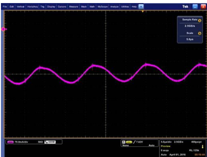
Figure 8: Input current waveform without any harmonic distortion
