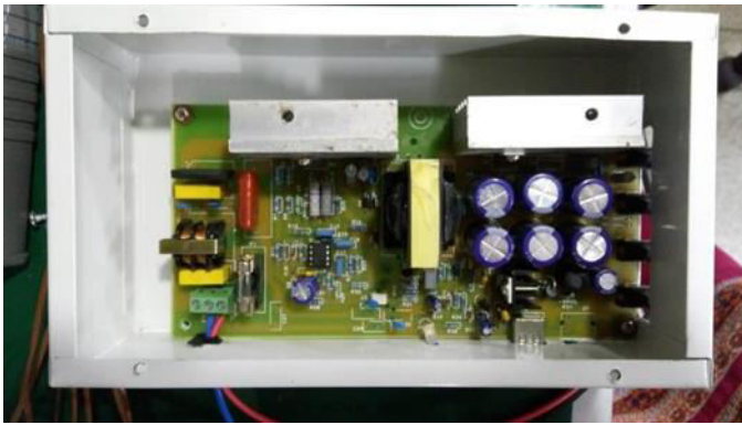
Figure 7: Hardware setup of the flyback converter
