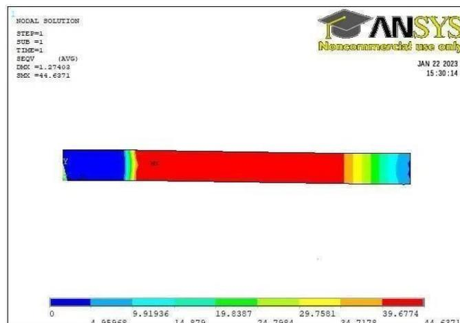
**Figure 3.2:** Max. Von Mises Stress of BFRC at 0 $^{\circ}$  Fiber Angle for Tensile
