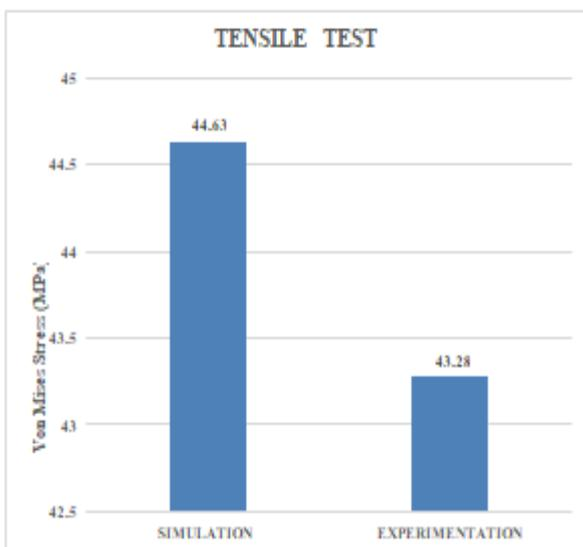
Figure 5.5: Simulation and Experimentation Von Mises Stresses at Optimum Fiber Angle of 0° for Tensile Test
