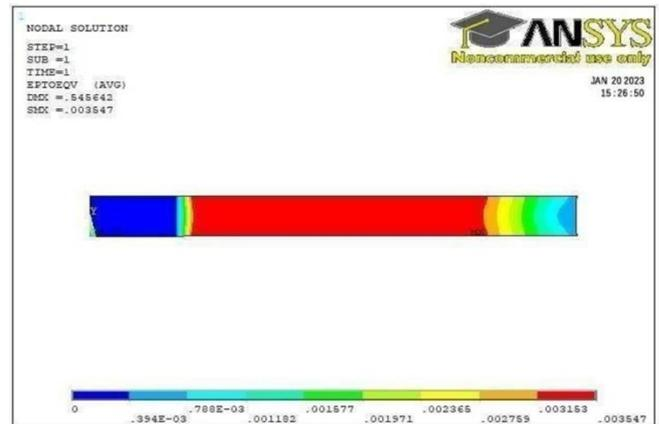
**Figure 3.3:** Max. Von Mises Strain of BFRC at 0 $^{\circ}$  Fiber Angle for Tensile Test
