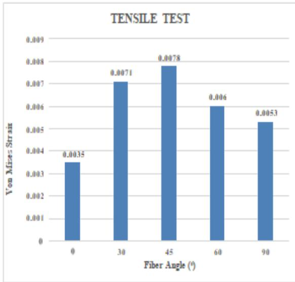
Figure 5.3: Simulation Von Mises Strains at Various Fiber Angles for Tensile Test
