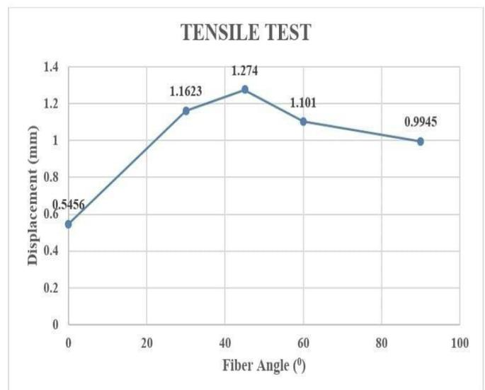
Figure 5.1: Simulation Displacements at Various Fiber Angles for Tensile Test
