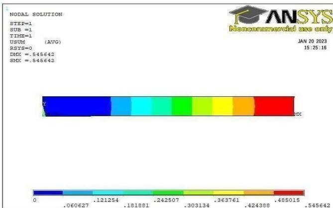
**Figure 3.1:** Max. Displacement of BFRC at 0 $^{\circ}$  Fiber Angle for Tensile test
