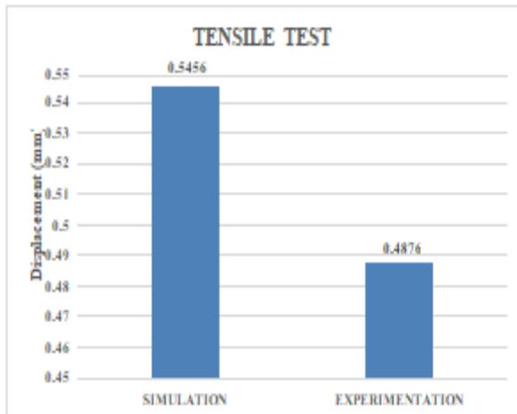
Figure 5.4: Simulation and Experimentation Displacements at Optimum Fiber Angle of 0° for Tensile Test
