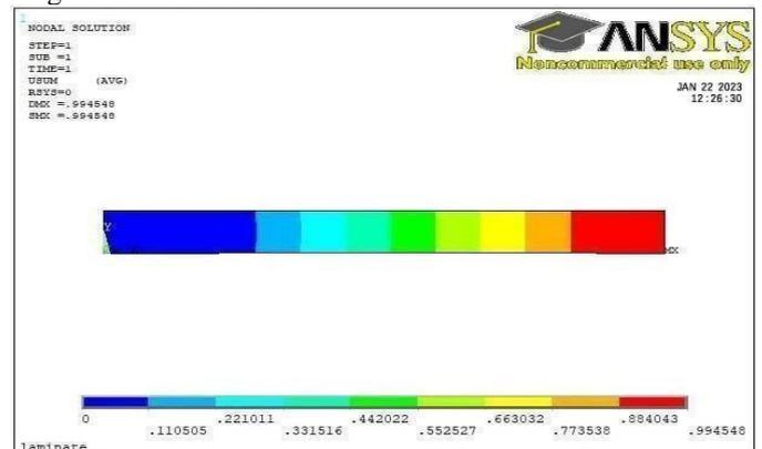
**Figure 3.4:** Max. Displacement of BFRC at 90 $^{\circ}$  Fiber Angle for Tensile Test
