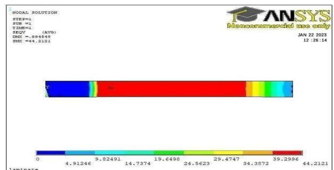
**Figure 3.5:** Max. Von Mises Stress of BFRC at 90 $^{\circ}$  Fiber Angle for Tensile Test
