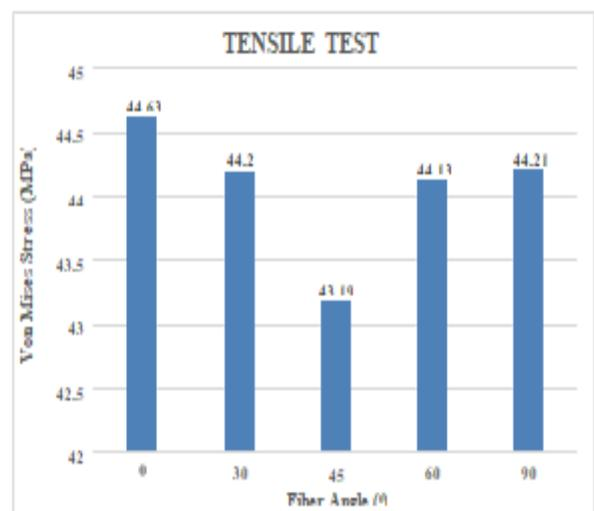
Figure 5.2: Simulation Von Mises Stresses at Various Fiber Angles for Tensile Test
