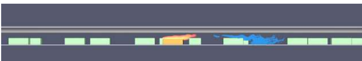
Fig. 29. First sprinkler activation at 136 s, illustrating tunnel conditions at initiation.
