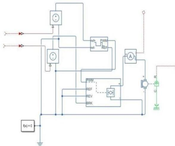
Figure 3.4: Motor Circuit and Controller Subsystem
