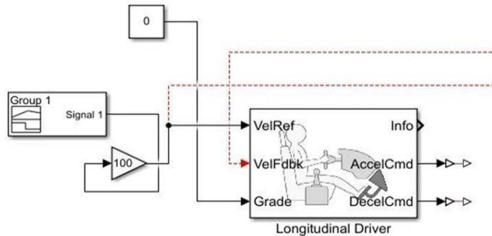
Figure 3.5: Driver Input Subsystem
