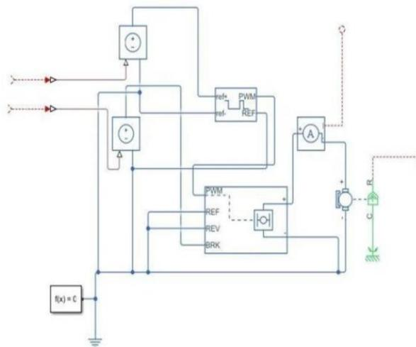
Figure 3.4: Motor Circuit and Controller Subsystem
