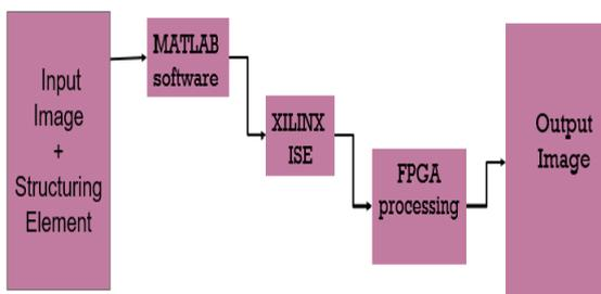
Figure 3: Basic steps for Processing of an Image
