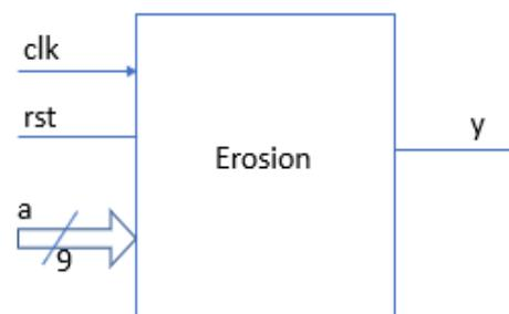
Figure 7: Block diagram of Erosion Operation
