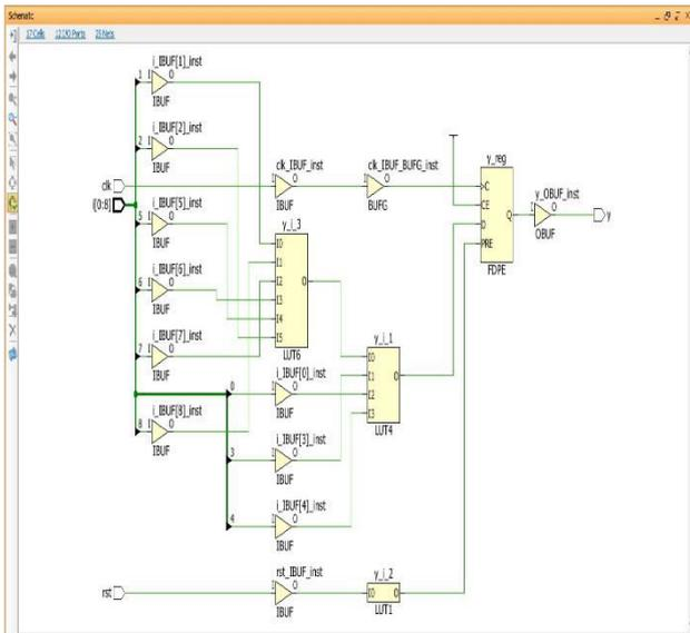
**Figure 8 : Synthesis Result of Erosion Operation**
