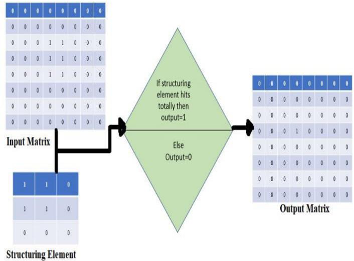
Figure 6 : Design model for Morphological Processing-Erosion
