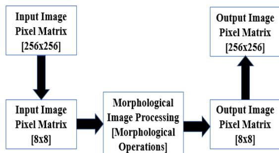
**Figure 2: Block diagram of Morphological Image Processing**
