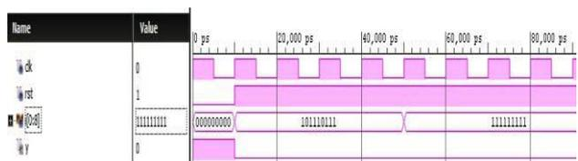
**Figure 11 : Simulation Result of Erosion Operation**
