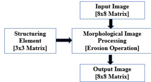
Figure 4: Block diagram of Morphological Image Processing with Erosion
