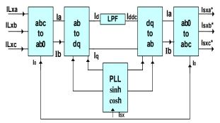
Fig.2 Block diagram of Synchronous reference frame (SRF) method
