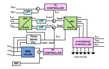
Fig 3 Synchronous Reference Frame Control Strategy
