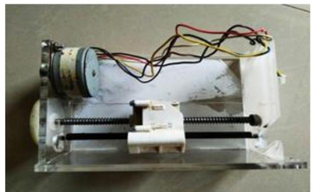
Syringe is placed on the socket of syringe pump. The plunger moves reverse and forward with sufficient pressure. Those pressure push the syringe for define time of dosage. Plunger relates to helix, which unify the plunger direction. The whole system is connected to simple gear system operated by stepper motor. Thus, stepper motor is connected to driver circuit. A driver circuit is used to control stepper motor driving speed.
