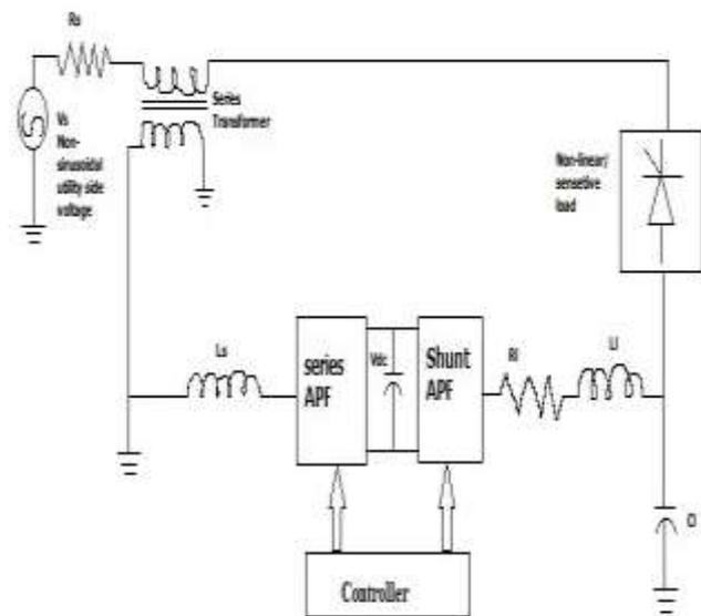
Fig. 1. Typical Structure Of Single Phase To Three Phase UPQC
