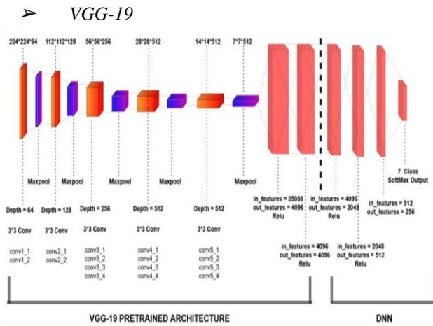
Figure 4: Modified VGG-19 Architecture
