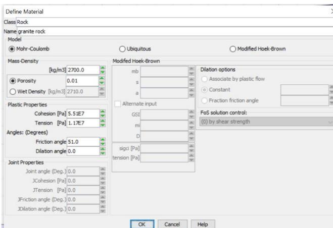
Fig - 3: Rock Slope materials' properties (Mohr-Coulomb)
