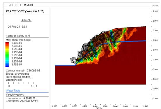
Fig - 12: Model 3 with both water table and pseudostatic force
