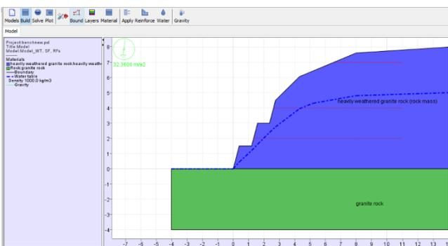
Fig - 9: Model 5, rock slope with water table, pseudostatic force and reinforcements
