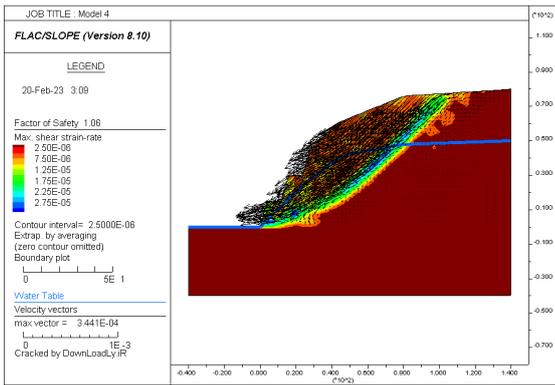
Fig - 14: Model 4 both water table, pseudostatic force and geogrids
