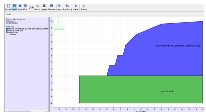
Fig - 5: Model 1, indicating the type of rock slope materials
