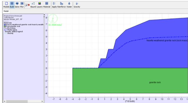
Fig - 7: Model 3, rock slope with water table and pseudostatic force
