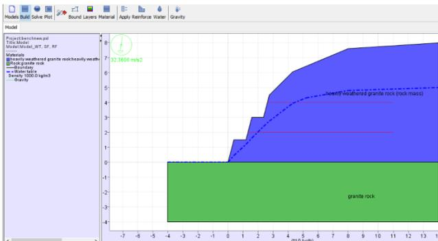
Fig - 8: Model 4, rock slope with water table, pseudostatic force and reinforcements
