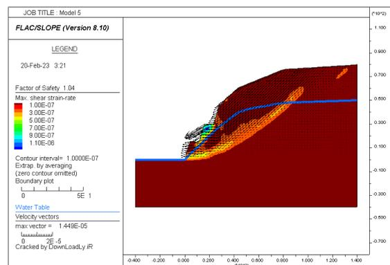
Fig - 13: Model 5 both water table, pseudostatic force and geogrids
