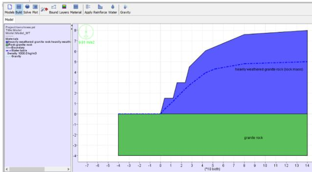
Fig - 6: Model 2, rock slope with the presence of water table
