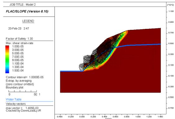
Fig - 11: Model 2 with water table and no pseudostatic force
