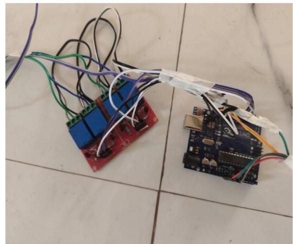
Fig. 5. Controlling system using Arduino
