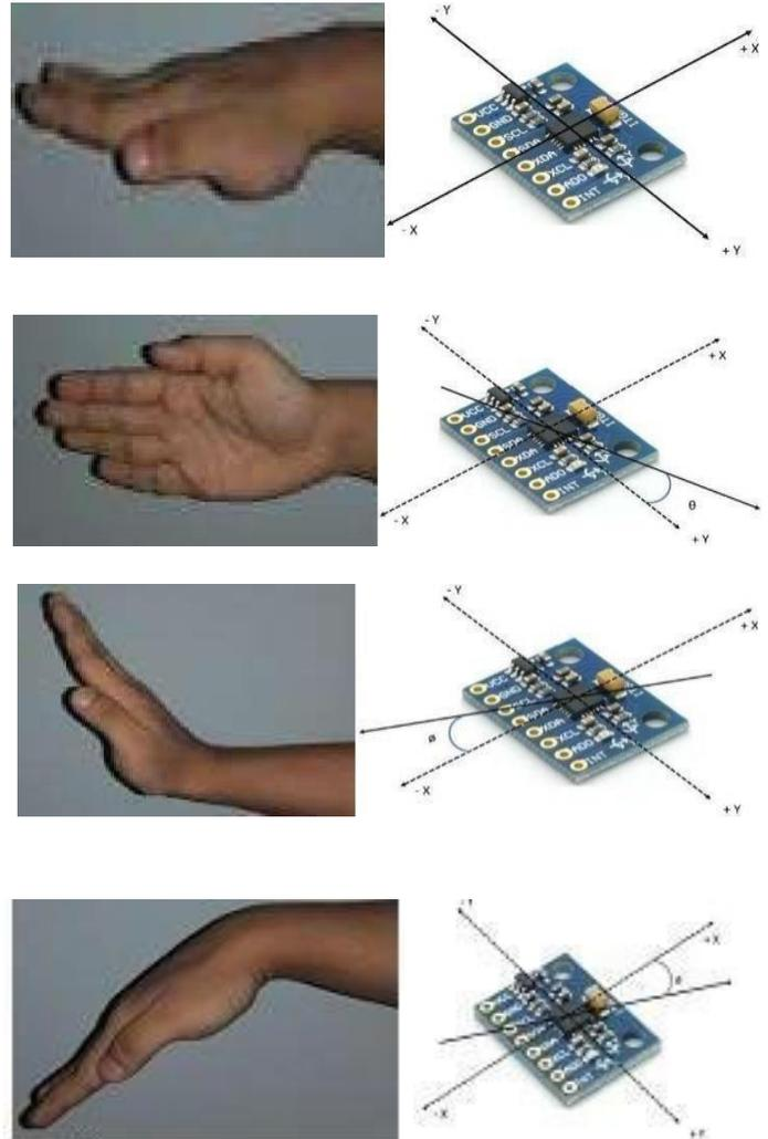
section must be designed and executed independently. An accelerometer is used as the sensor to detect the tilting of the hand, which in turn transmits the signals through the RF modules.
