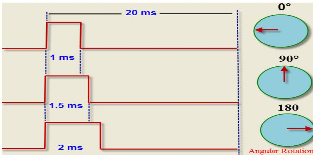
Figure 5 CONTROLLING A SERVO WITH ANGLE ROTATIONS
