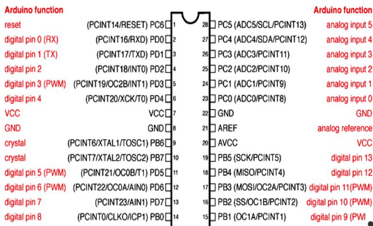
Digital Pins 11, 12 & 13 are used by the ICSP header for MOSI, MISO, SCK connections (Atmega168 pins 17, 18 & 19). Avoid low-impedance loads on these pins when using the ICSP header.
