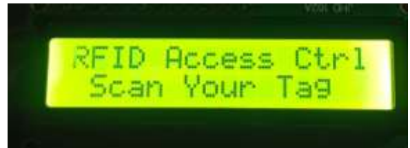
Fig 1.6 LCD display to indicate the scanning process
