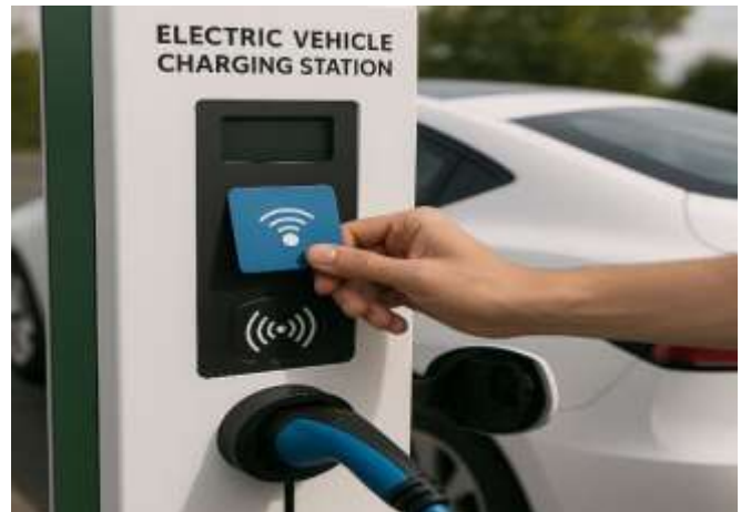
Fig -1: Smart Electric Vehicle Charging Station Using RF-ID
