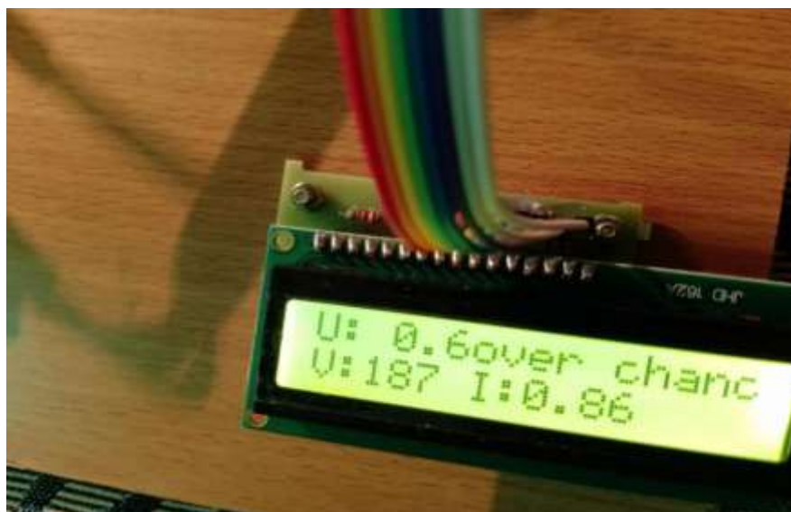
Fig. 6: LCD Display Showing Voltage, Current, and Power Readings
