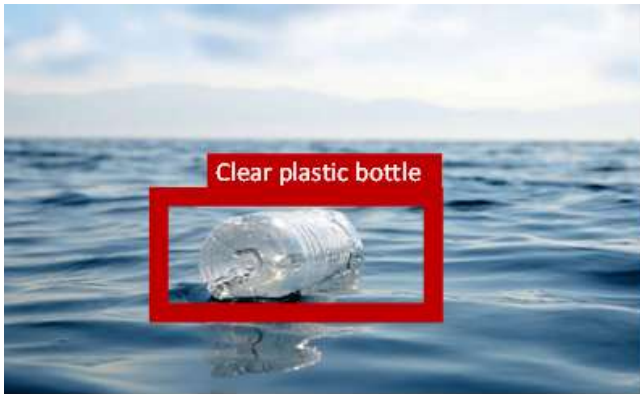
Fig. 5. Sample output of the proposed YOLO-based system detecting a floating plastic bottle with bounding box and class label.
