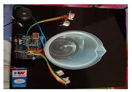
The above picture represents the working of the smart bin with the all requirements attached to it. When the garbage is thrown outside the bin then the buzzer win give the warning.
