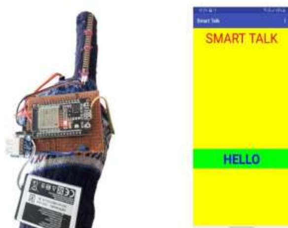
Figure 7 Smart Glove Gesture for Hello
