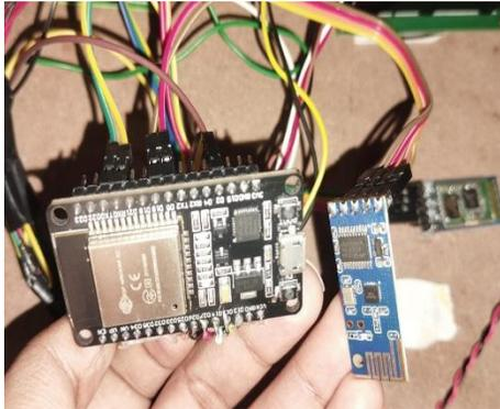
Fig 5: ESP32 module to XBee RFX240 module
