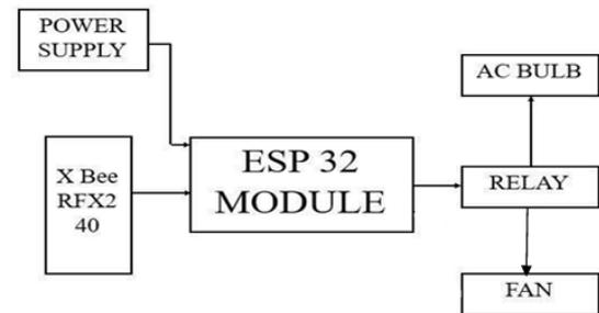
Fig.2: Block diagram of Receiver of Smart Gloves for Blind, Deaf and Dumb Using Sign and Home Automation Mode.
