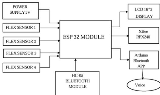
Fig.1: Block diagram of Transmitter of Smart Gloves for Blind, deaf and Dumb Using Sign and Home Automation Mode.
