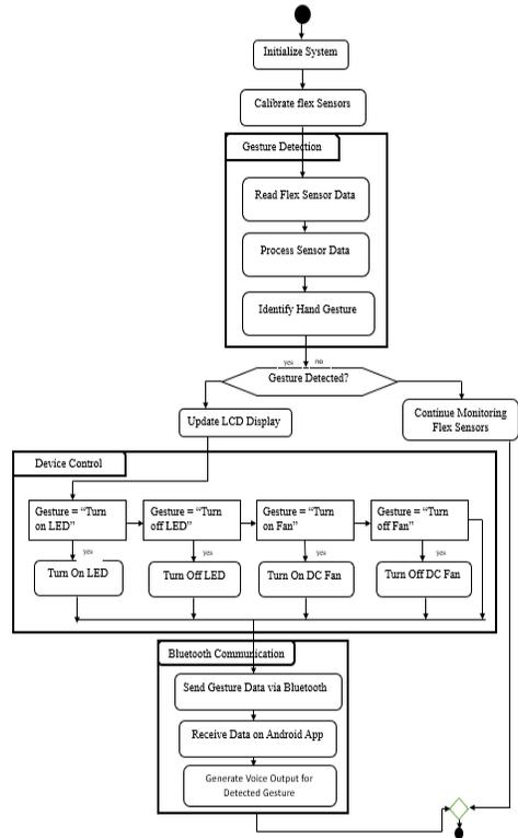
Fig. 3: Flow Chart of Smart Gloves for Blind, Deaf, Dumb Using Sign & Home Automation Mode
