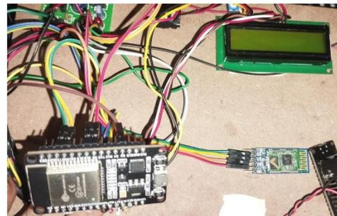
Fig 5: ESP 32 module to LCD Display
