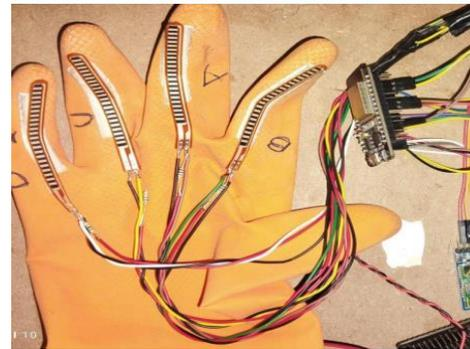
Fig 4: Flex sensor to ESP 32 Module
