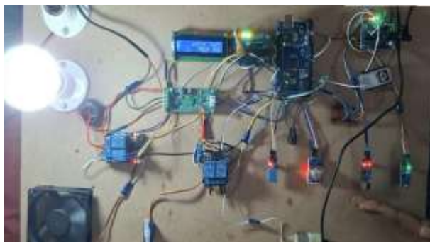
Fig.3: Automatic Lighting Using LDR and IR Sensor
