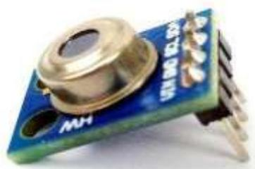
Fig. 2. MLX90614 temperature sensor
