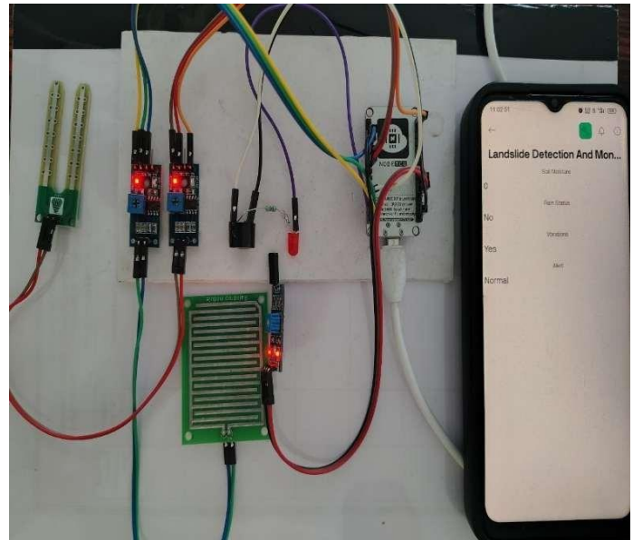
Fig. Sensor and Blynk IoT application Dashboard without any sensor input
