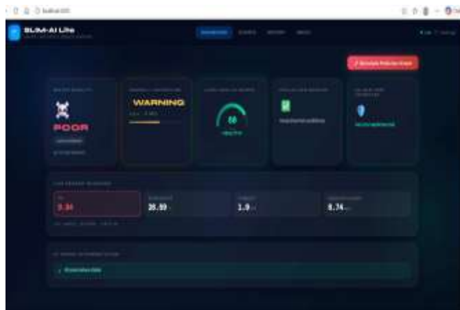
Figure 5.2: Dashboard showing a detected pH anomaly
