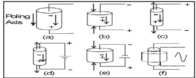
Fig 4:- Effect of different direction of applied stress or charge
