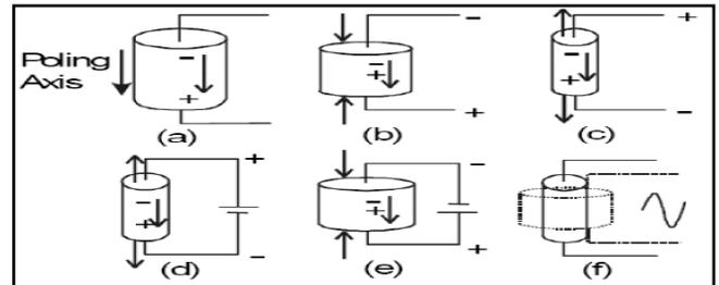
Fig 4:- Effect of different direction of applied stress or charge
