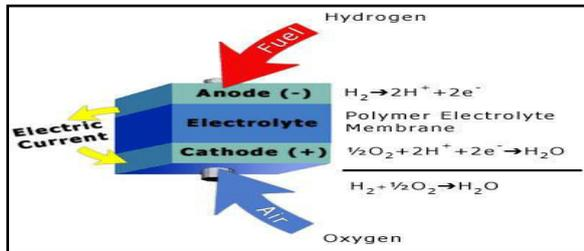
Fig. 7:- Fuel cell system with conducting polymer
