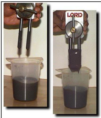
**Fig:- 2** :M.R. fluid in working
