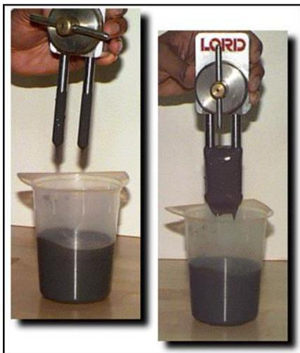
**Fig:- 2** :M.R. fluid in working
