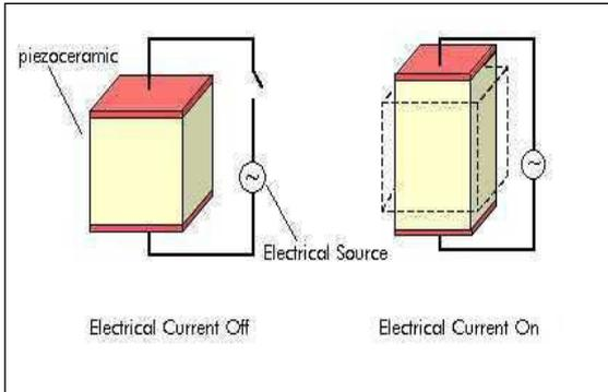
**Fig:-1** Piezoelectric effect.
