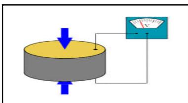
Fig 3:- Converse piezoelectric effect
