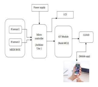
The medical box is provided with two IR sensor which detect the intake of medicine as well as detect if the box is empty. It is then interlinked with the microcontroller. Here we use Arduino UNO as the microcontroller. This can be run via both power supply as well as using battery.
