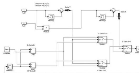
( Implementation of P&O MPPT algorithm in Simulink using if-else blocks)
