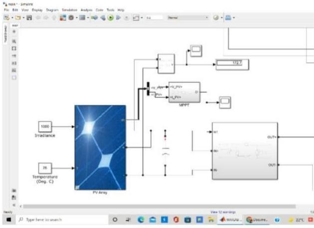
( Simulink model of PV based DC system P )
