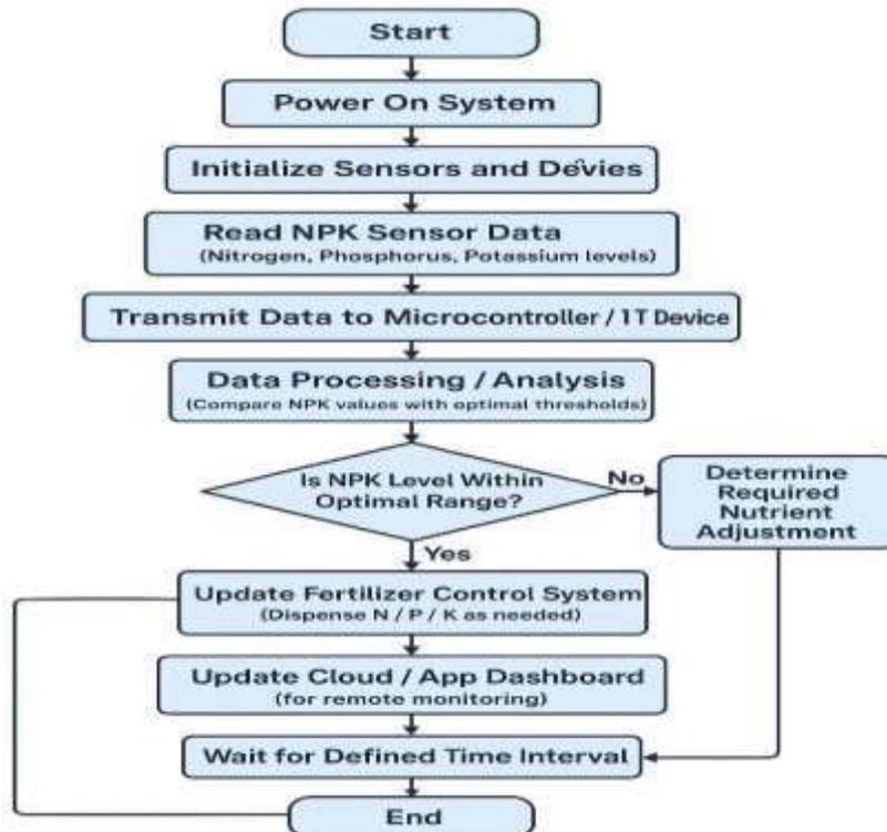
**Fig 1:** The flowchart represents the working process of a Smart NPK Monitoring and Control System for Precision Agriculture
