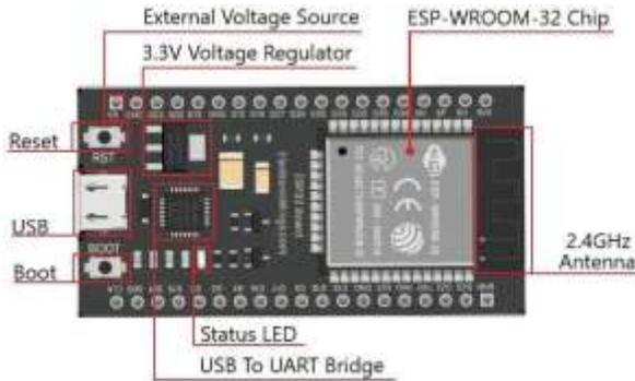
**Fig 2:** ESP 32 Board highlights
