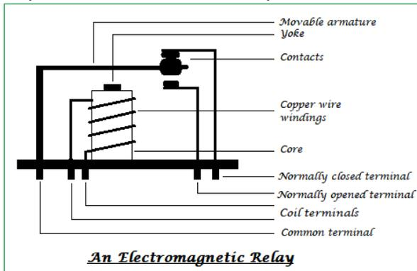
Fig 5: An electromagnet relay
