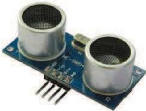
Figure 2.3.3: Ultrasonic Sensor
