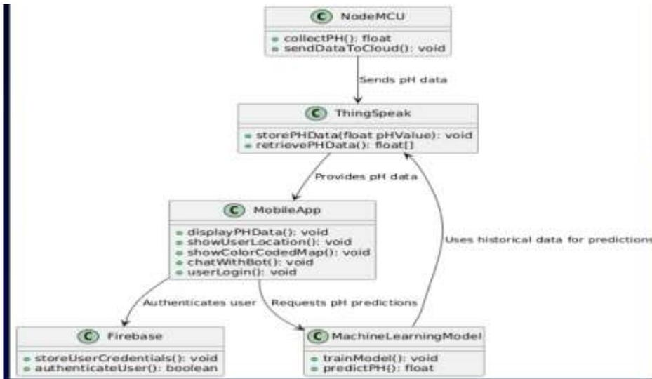
FIGURE 1. System Architecture for Smart pH App
