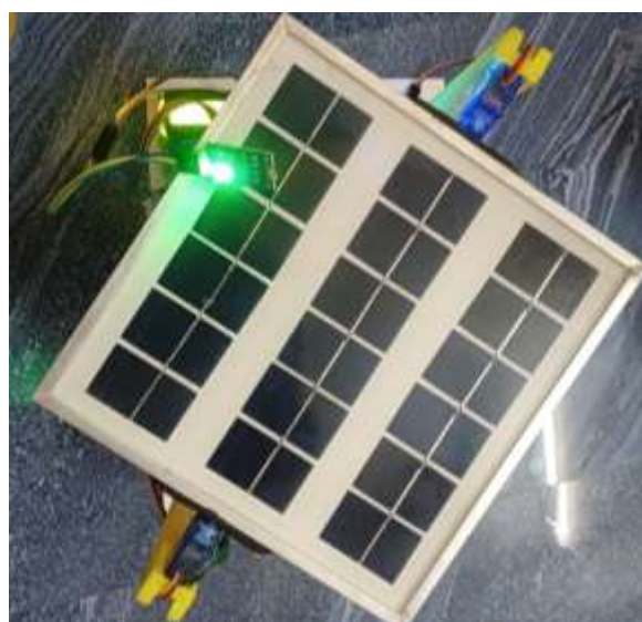
Fig 4: LDR-controlled servo aligned the solar panel in sunlight
