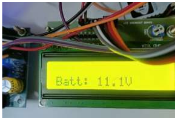
Fig 3: Battery voltage detects using voltage sensor and monitoring in LCD
