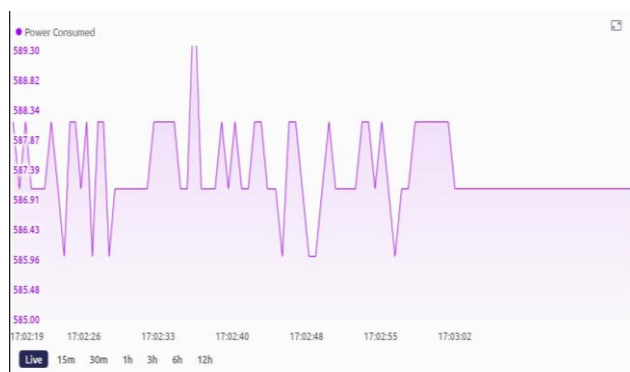
Fig.13 Blynk superchart for the visualization of the consumed power
