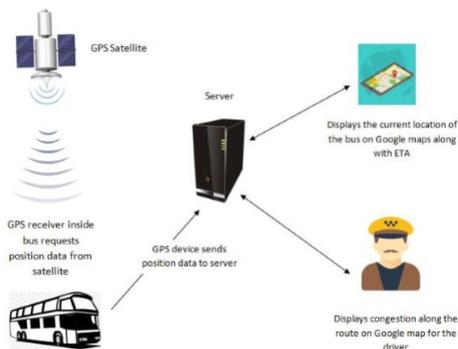
Fig 1. Bus Tracking Architecture
