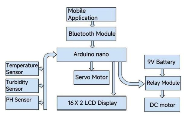
In the proposed system, the sensors such as pH, turbidity, temperature and humidity are connected to the core controller as shown in figure 1. To transfer the data over the internet, the core controllers access the sensor values and process them. The Arduino Nano is used as a core controller. The sensors are also connected to the ESP8266 Wi-Fi module to display the data on the IOT Adafruit server.
