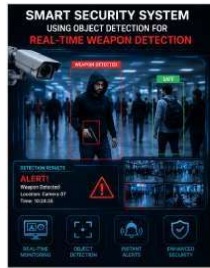
Fig. 3. Real-time weapon detection output. The system flags the armed individual with a red “WEAPON DETECTED” bounding box while the unarmed individual nearby is marked “SAFE” in green. The alert panel logs the event (camera ID, timestamp) and raises an immediate visual alarm, consistent with the recall-focused behaviour of Model B.
