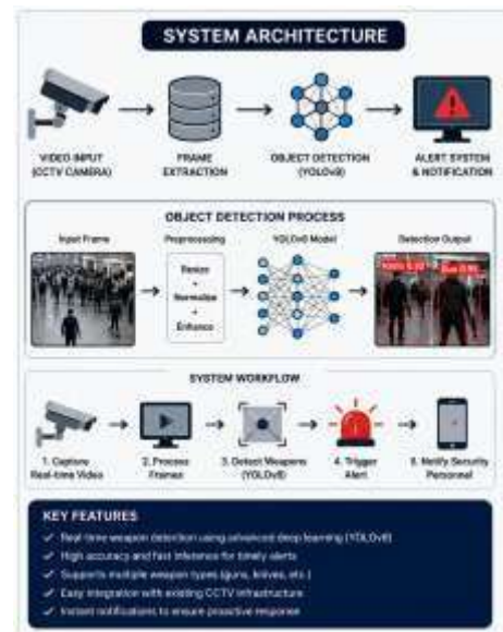
Fig. 1. System architecture: video is captured from a CCTV camera, frames are extracted and preprocessed (resize, normalize, enhance), passed through the YOLOv8 model for object detection, and matched detections trigger the alert system, which notifies security personnel in real time.
