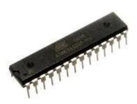
The Atmel ATmega8A is a low-power CMOS 8-bit microcontroller based on the AVR enhanced RISC architecture. By executing powerful instructions in a single clock cycle, the ATmega8A achieves throughputs close to 1MIPS per MHz. This empowers system designer to optimize the device for power consumption versus processing speed.
