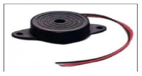
The piezo buzzer products sound based on reverse of the piezoelectric effect. The generation of pressure variation or strain by the application of electric potential across a piezoelectric material is the underlying principle. These buzzers can be used alert a user of an event corresponding to a switching action, counter single or sensor input. They are also used in alarm circuits
