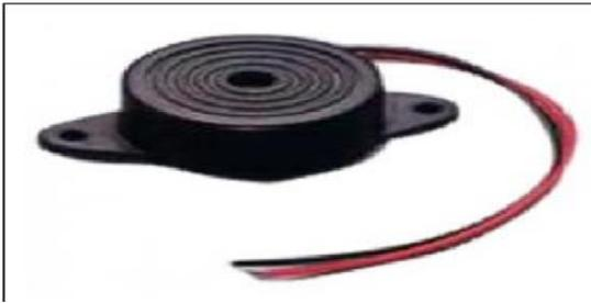
The piezo buzzer products sound based on reverse of the piezoelectric effect. The generation of pressure variation or strain by the application of electric potential across a piezoelectric material is the underlying principle. These buzzers can be used alert a user of an event corresponding to a switching action, counter single or sensor input. They are also used in alarm circuits
