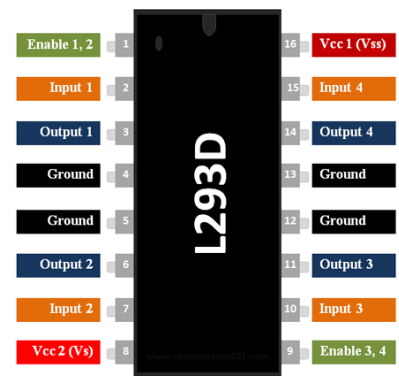
Fig 4 L293D motor driver IC
