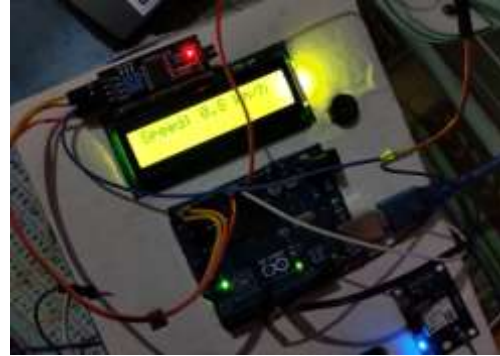
Fig -9 Over-speed monitoring system
