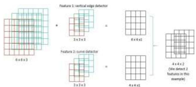
Fig. 1. Convolution using multiple filters [2]
